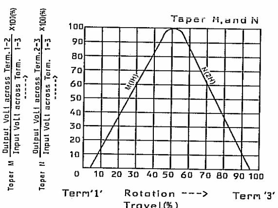
NOTE: Resistance characteristic of curve N is plotted with respect to terminal '3'
